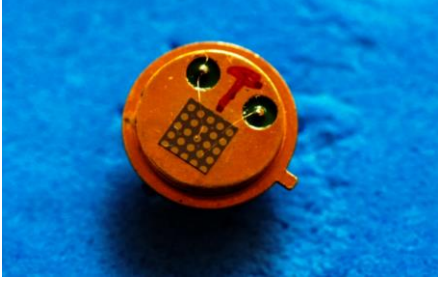
Fig. 2. 0.5 mm dia diodes for DLTS and irradiation analysis
